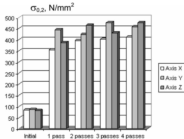
Figure 2. Conventional yield strength of copper M1 at compression versus the number of ECAP passes (route B<sub>C</sub>) at room temperature.
