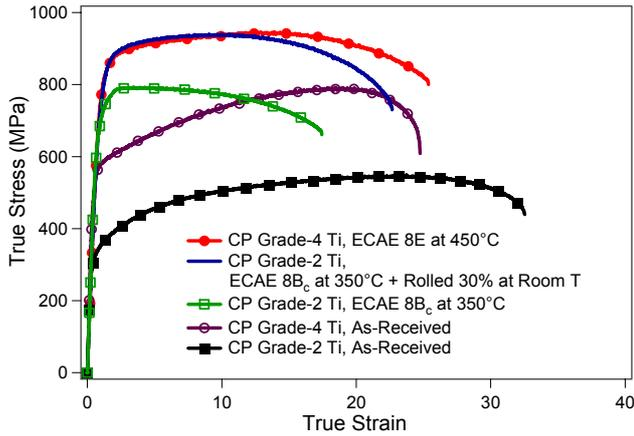
Figure 1. Room temperature tensile true stress vs. true strain response of the ECAE processed CP Grade 2 and Grade 4 Ti and ECAE plus cold-rolled CP Grade 2 Ti
