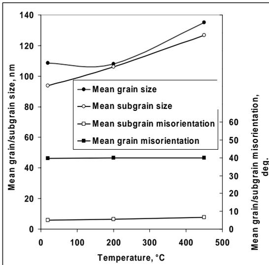
Figure 1. Mean grain/subgrain size and mean misorientation angle as a function of annealing temperature in HPT-processed Armco iron
