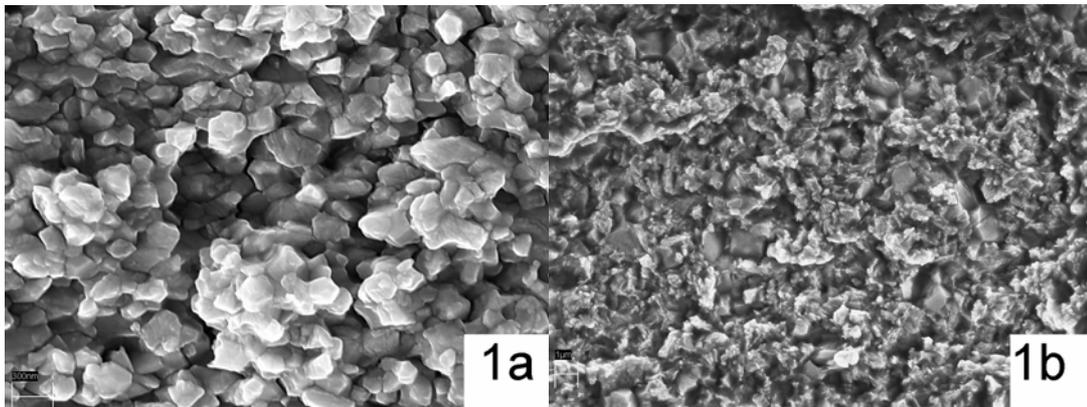
*Figure 1. Comparison of the fatigue fracture surfaces of ultrafine-grained and microcrystalline Nickel*
