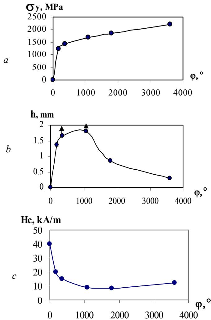
Figure 1. Mechanical and magnetic properties of the Fe-15%Co-25%Cr alloy upon bending tests. The variation of (a) the yield strength  $\sigma_y$ , (b) ultimate bending flexure  $h$ , (c) coercivity  $H_c$  as function of the angle  $\varphi$  of rotation of mobile anvil. Arrows ( $\uparrow$ ) correspond to samples that not fail upon bending.
