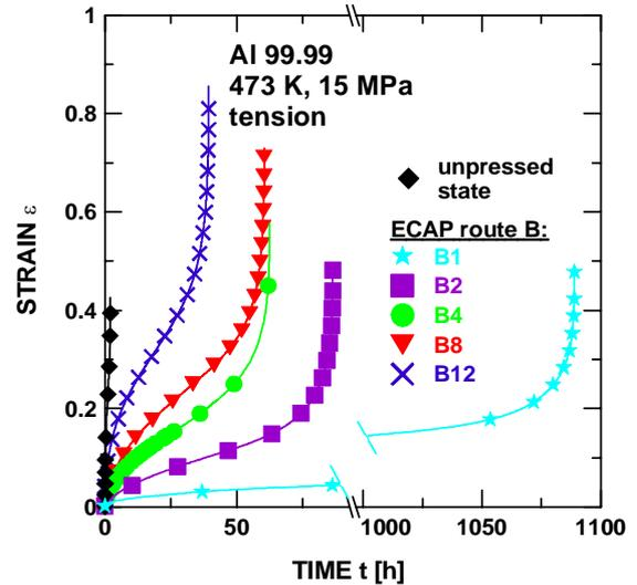
Figure 1. Effect of the number of passes on the creep life
