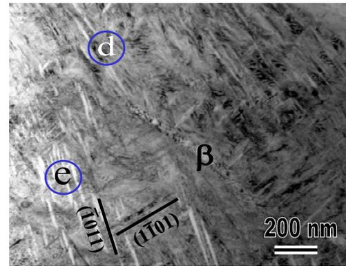
Figure 2. Deformation twins observed in Ti-6Al-4V after two ECAE passes at 800°C following route A.
