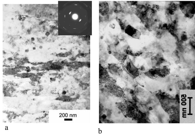
Figure 1: Bright field images of the Al 6061 alloy microstructure after ECAP: (a) at 50 °C with back pressure, 1 pass, (b) at 110 °C, 4 passes
