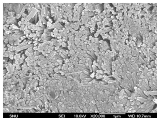
Figure 1. SEM-image of the UV-irradiated film surface
