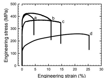
Figure 2. Engineering stress – strain curves for the Al 6061 alloy after ECAP (a) at 50 °C, with back pressure and 1 pass, (b) at 110 °C, 4 passes, (c) conventional T6 heat treatment and (d) solution treatment and quenching
