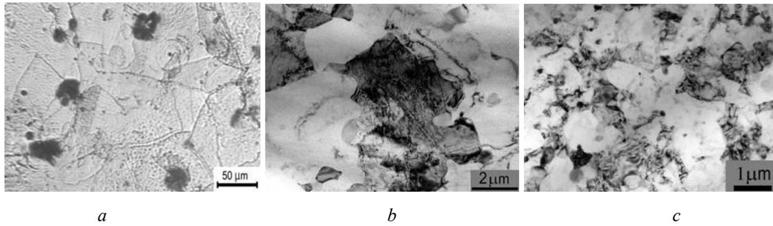
Figure 1. Microstructure after: a – annealing, b – ECAP, c - HPT
