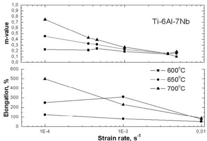
Figure 1. Dependence of relative elongation and strain rate sensitivity coefficient  $m$  on strain rate and temperature for UFG Ti-6Al-7Nb
