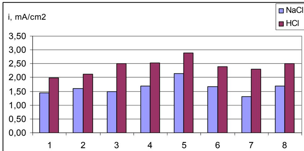
Figure 1. Corrosion current density in 3% NaCl and 1M HCl solutions. 1-A1, 2-A2, 3-A4, 4-A8, 5-A12, 6-B12, 7-F12, 8-CG Cu
