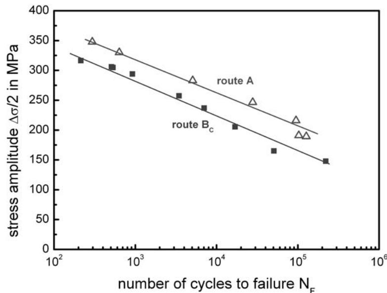
Figure 1. Wöhler (S-N) plot of UFG AlMg1.5 after 8 ECAP passes with ECAP route A and B<sub>c</sub>
